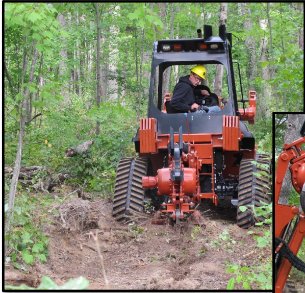
Vibratory plow creates a trench to cut root grafts in an effort to prevent the spread of oak wilt
