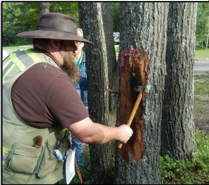
Removing the bark to examine old pressure pads
