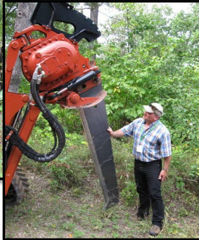
Vibratory plow creates a trench to cut root grafts in an effort to prevent the spread of oak wilt
